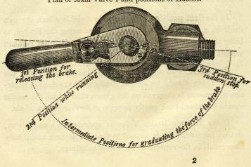
In the first position, a free communication is formed through the large ports, a, a, in the valve 1, from the Main Reservoir to the Brake Pipe; but
