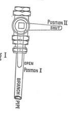
Fig. II. A three-way tap fitted on to the body of the triple valve. When the handle is vertical (Position I.) the quick-acting valve is in operation; when the handle is horizontal (Position II.) the triple valve works as on the ordinary brake gear; and when placed midway between (Position III.) the brake is cut off.
