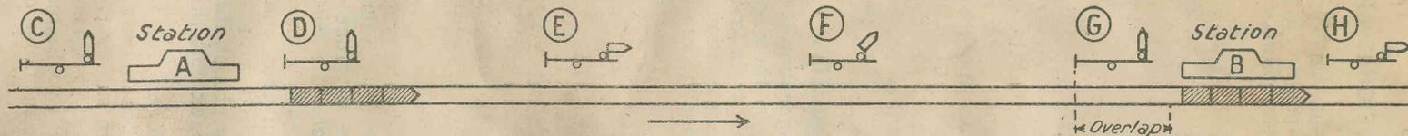
The above Diagram represents a series of Block Sections on which Automatic (Three-position) Signalling is in operation. The various Sections being C—D; D—E; E—F; F—G; and G—H.
