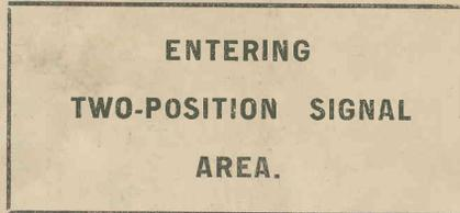
(b) The Fixed Signal (Interlocked or Automatic) at the entrance to a Section in which Two-position (Lower Quadrant) Signals are in operation will, provided the Section ahead is clear, display the Clear Signal although the Home Signal next in advance may be at Danger. It must be understood, however, that in such case the Signal next in advance is a Distant Signal, and Drivers must be prepared to act as prescribed in Regulation 55, in the event of the Distant Signal being at Danger.
