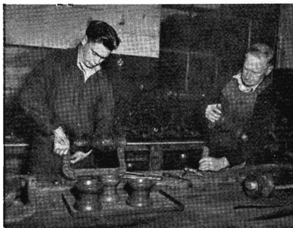
Repairing and assembling a set of catenary insulation in the Overhead Depot Workshops, at Batman-av. Defective insulation found by maintenance gangs is replaced.
