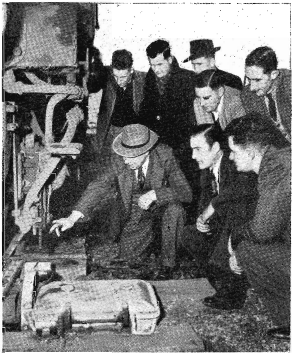
The functions of the tripping valve gear, with which all electric trains are equipped to prevent them passing a signal at danger, are being explained to a group of trainees at one of the instructional train's roadside stops.
