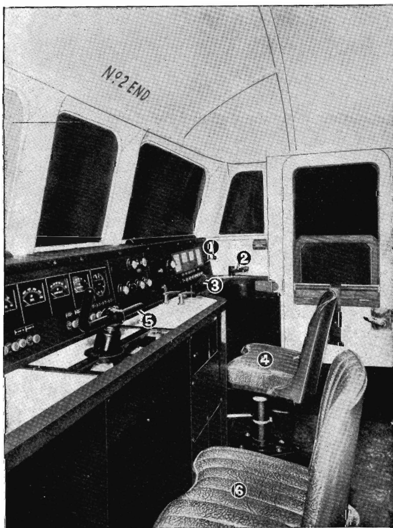
Interior of one of the driving cabs: (1) horn-operating lever, (2) vacuum brake control, (3) master controller, (4) driver's seat, (5) hand brake, (6) assistant's seat.
