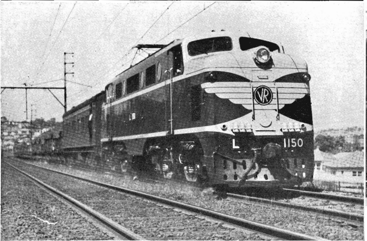
L. 1150's TEST : The first of the V.R.'s 25 2,400 h.p. electric locomotives, which will ultimately be used on the Gippsland line, commencing a recent test, from a standing start, up the 1 in 50 grade of the Glenroy Bank.
