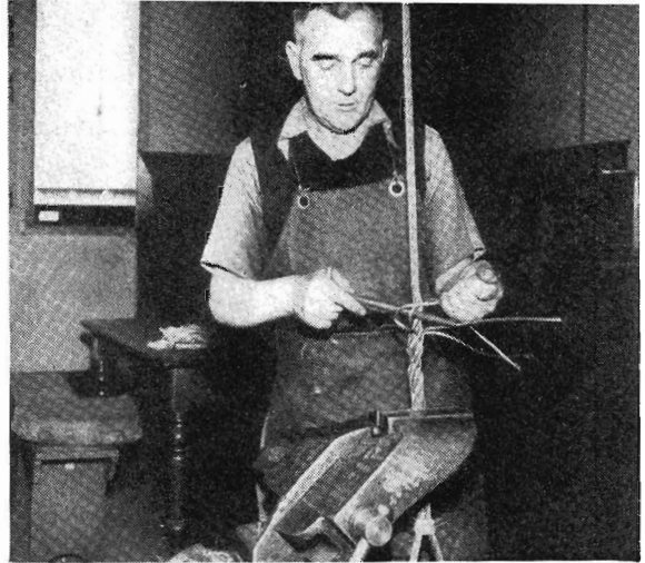
Rope Splicer C. Letham making a wire rope sling for use on one of the many departmental cranes.
