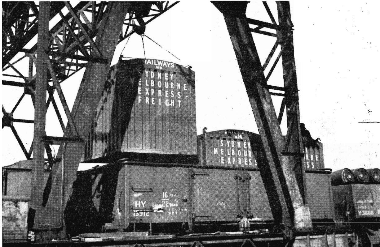
A truck containing three containers with freight from Sydney being unloaded by crane at Kirwan's Siding, Melbourne Yard. The containers have an approximate capacity of 320 cubic feet or 5\frac{1}{2} tons weight.
