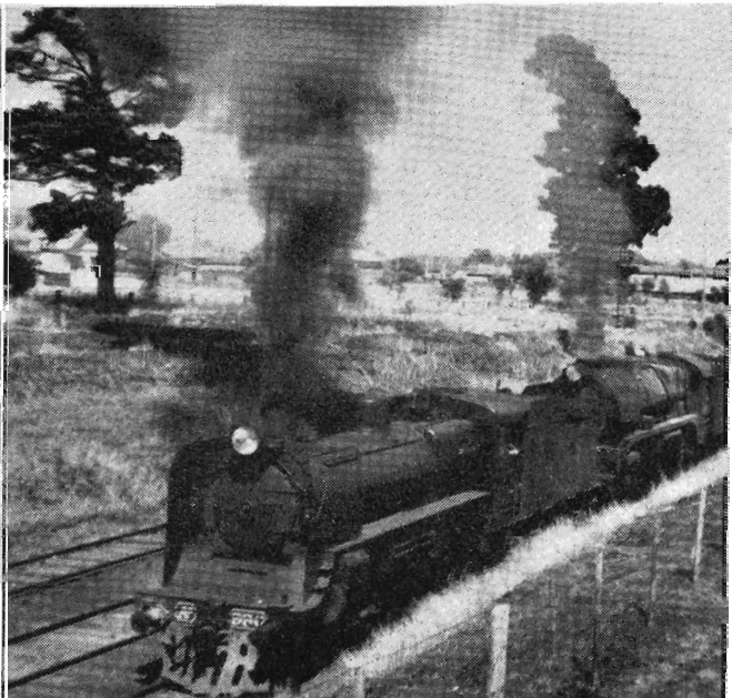
TRIPLE EFFORT: With a load of 1,220 tons, the A2 and R class locomotives leave Ballarat East to tackle the 1 in 50 grade of the Warrenheip.
