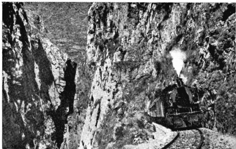
GOING UP: Passenger train in typical mountain scenery, Central Railway of Peru. This railway crosses the main range of the Andes at an altitude of 15,800 feet. There are 59 bridges, 66 tunnels and 21 zigzags. Half the main line, which is 4 ft. 8½ in. gauge, is curved track sometimes with a radius as low as 100 metres. Maximum gradient is 1 in 23 uncompensated for curvature, and there are long stretches of 1 in 25.
