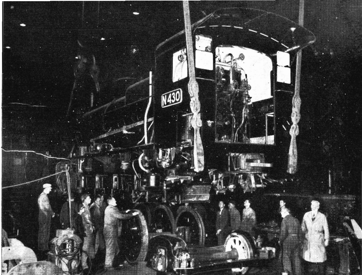
Wheeling an N class locomotive at Newport Workshops. A powerful overhead electric crane is used for hoisting locomotives to enable their wheels and axles to be rolled in.
