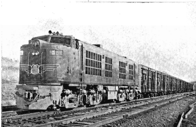
NEW POWER: The first of ten 4,500 h.p. gas-turbine-electric locomotives, ordered by the Union Pacific Railroad, hauling a freight train. The locomotive weighs 248 tons and has a starting tractive effort of 135,000 lb. It burns heavy oil.
