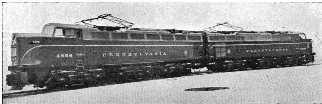
U.S.A.: Pennsylvania Railroad's rectifier locomotive with 2 (Bo-Bo-Bo) wheel arrangement. Two units are coupled to form a 6,000 h.p. locomotive. They are suitable for existing low frequency or for industrial frequency single phase systems.
