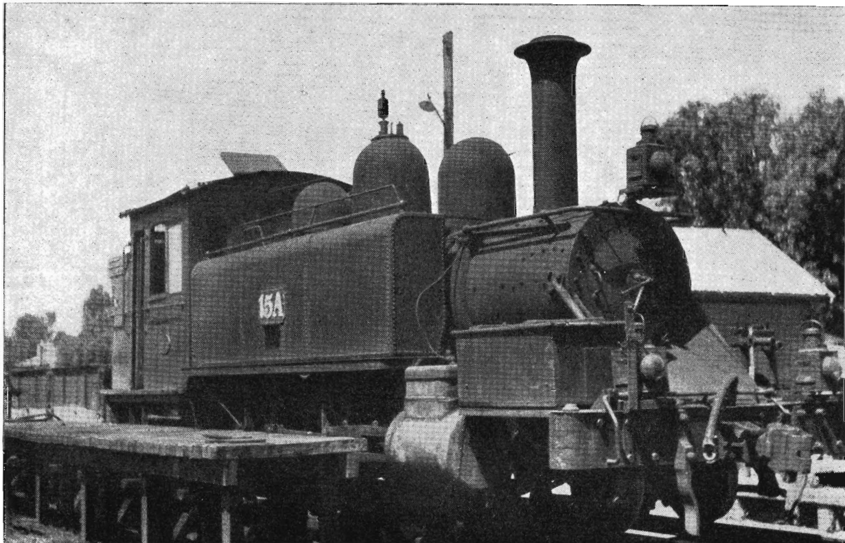
The narrow gauge line locomotive NA 15 at Wangaratta. It was one of the last of the class built in 1915 at Newport Workshops.
