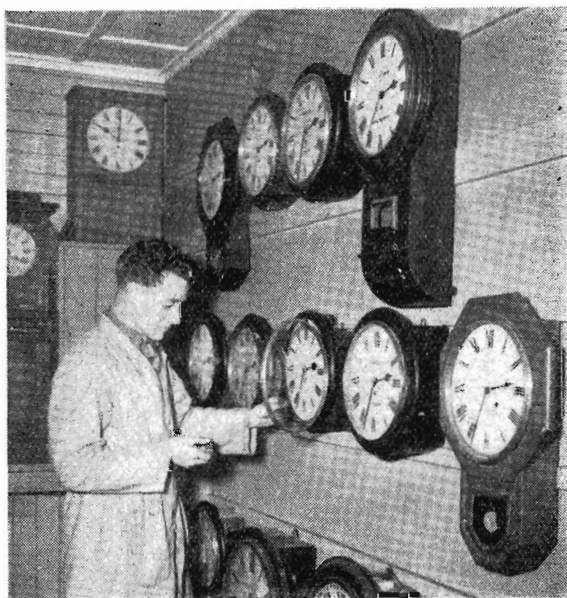
Synchronising clocks after repair and adjustment prior to issue to stations and depots.
