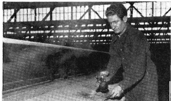
Removing old paint from the wing roof of a passenger car at North Melbourne Workshops.
