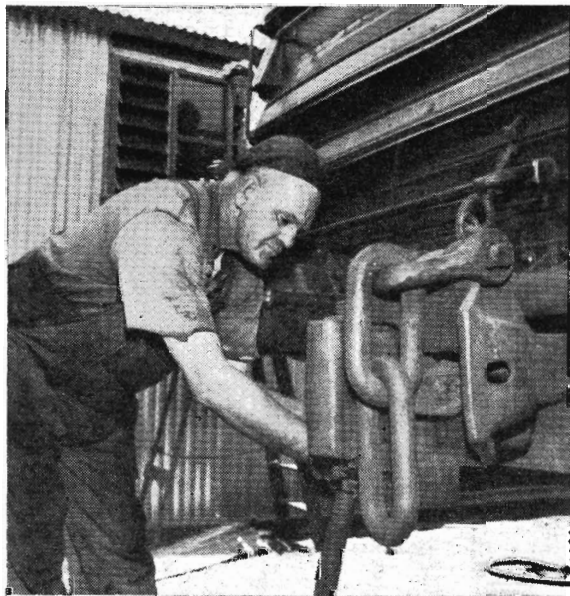
Mr. Dunstan fits a hose pipe on louver truck.
