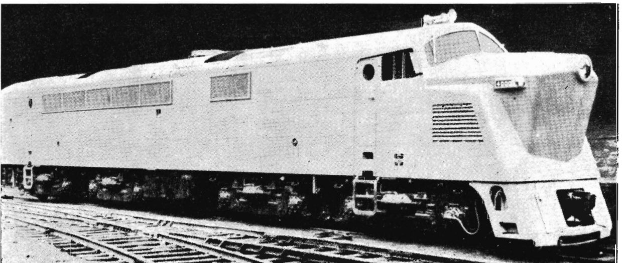
The Baldwin-Westinghouse 4,000 h.p. gas turbine passenger locomotive. It was built as an experiment with full realization that intensive development would be necessary before it could become a commercial product. The locomotive is in one unit, arranged as a single-end operation, and is carried on four two-axle swivel bogies, giving a B-B-B-B arrangement.
