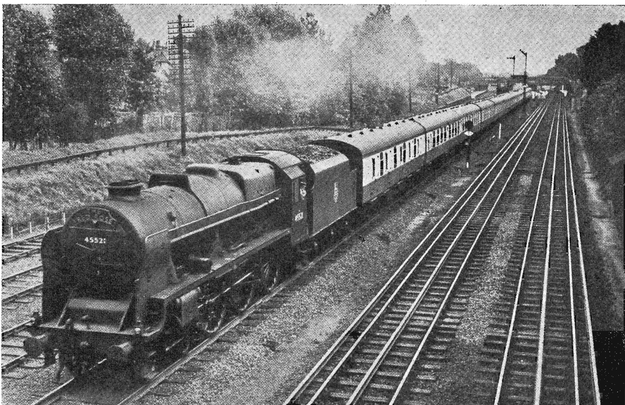
One of British Railways named expresses, Red Rose , near Hatch End, Middlesex. Hauled by a Patriot class 4-6-0 locomotive, it covers the 193½ miles from Euston to Liverpool Lime-st. in 3½ hours non-stop.
