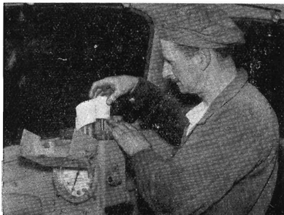
Removing the speed recorder chart in the cabin of a diesel-electric locomotive so that a check can be made.
