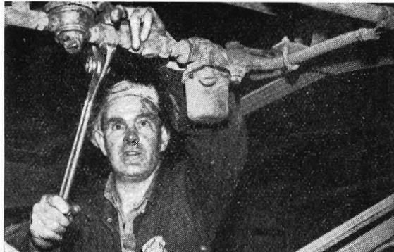
Assembling the airline to the watering system of a rail-car.
