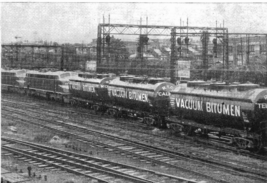
HOT TRAFFIC: Fast goods leaving Melbourne Yard for Adelaide with three of the Vacuum Oil Company's insulated tank cars for the carriage of hot bitumen. Preheated at Altona to about 400°F., the bitumen arrives in Adelaide, 23 hours later, hot and ready for immediate use. The tank cars have been named after famous road builders: McCormick, Calder, Telford, Macadam, R. M. Smith and Callaway.
