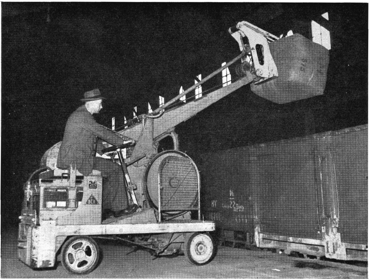
Bale-stacking truck makes wool loading easy.
