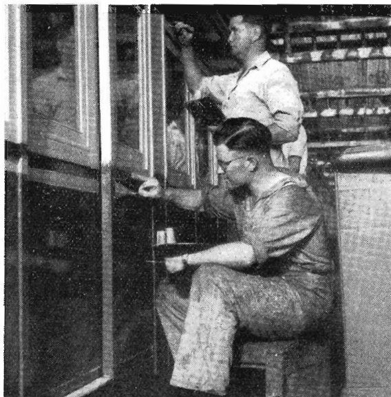
Painters lining up the body of a suburban sliding-door car at Jolimont Workshops.
