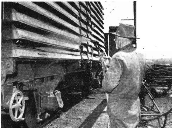
An air-controlled spray gun being used to repaint a louvre truck at Bendigo Workshops.
