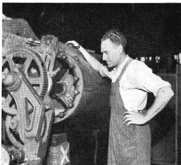
At work on locomotives : (left) Fitter N. Geddes and Fitter's Assistants C. Finlay and A. Speedy overhaul D3 619, and (right) Fitter's Assistant W. Mitchell bores out a D3 cylinder.
