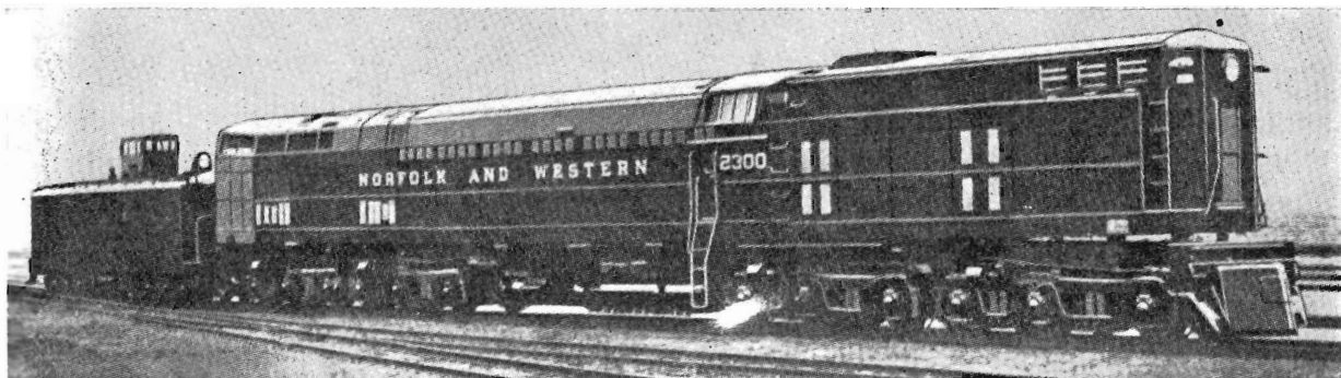
The Norfolk and Western's experimental coal-burning turbine-electric locomotive is rated at 4,500 h.p. and is designed for a maximum speed of 60 m.p.h. It has a maximum rated tractive force of 175,000 lb. and a continuous tractive force of 144,000 lb. at 9 m.p.h. There are four six-wheel trucks with each axle motorized.
