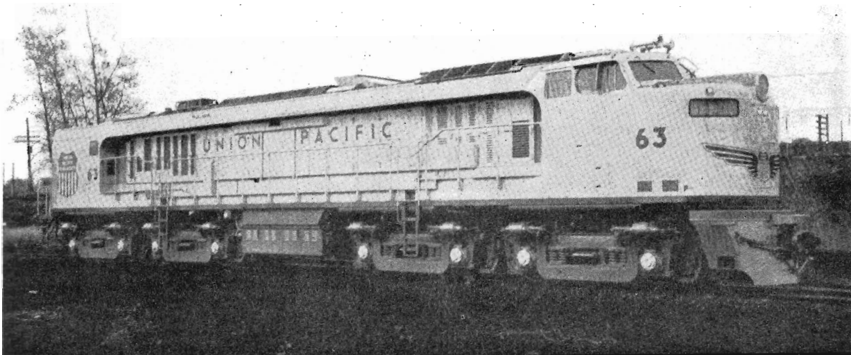
A modified unit, one of three recently delivered, of the Union Pacific's fleet of gas-turbine-electric locomotives. These locomotives have a starting tractive force of 135,000 lb. There are four four-wheeled trucks with each axle motorized. These locomotives burn heavy oil.
