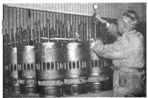
Checking the diameter of the bore of cylinder liners of the diesel engine with a mercer type gauge to get an indication of wear or distortion.
