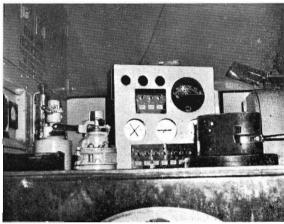
Driving instrument panel of the T class locomotive. On the right is the throttle handle, lower left the automatic brake handle, and at upper left the independent brake handle.
