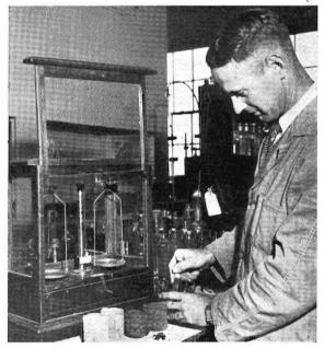
Checking the quality of briquettes used in locomotive water
