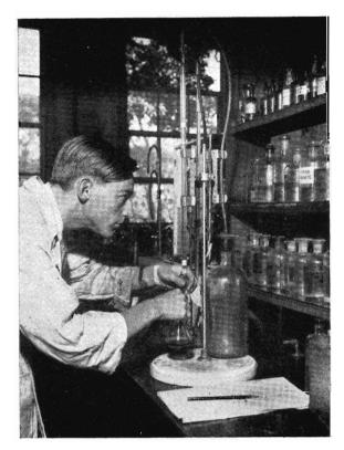
Instrument used for determining the amount of dissolvedj solids in water.
