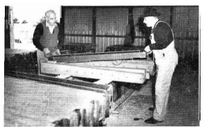
Stripping moulds from finished fence posts.
