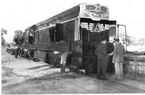
The end of the operation. The locomotive has been lowered on to its Victorian bogies and the gantry removed.
