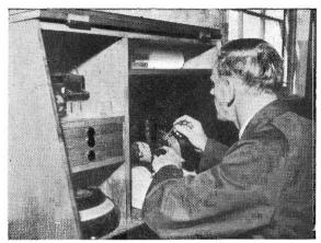
Using an absorptiometer (sensitive light absorption meter) to obtain the metal content of oil from a diesel crank-case.
