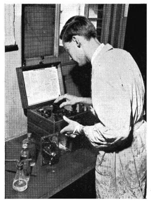
Equipment for analysing water and determining its hardness.
