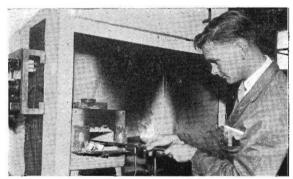
Furnace used for burning oil for determination of ash content of oil from diesel crank case.
