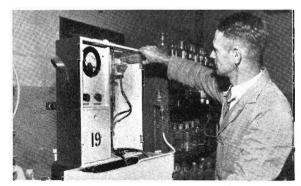
In this instrument water is tested for the relative activity of basic or acid reaction.
