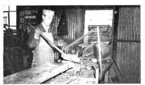
Straightening and cutting reinforcing wire.
