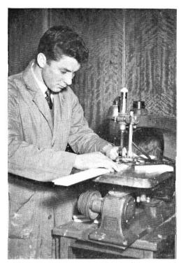
Cutting out lettering with the jig saw.
