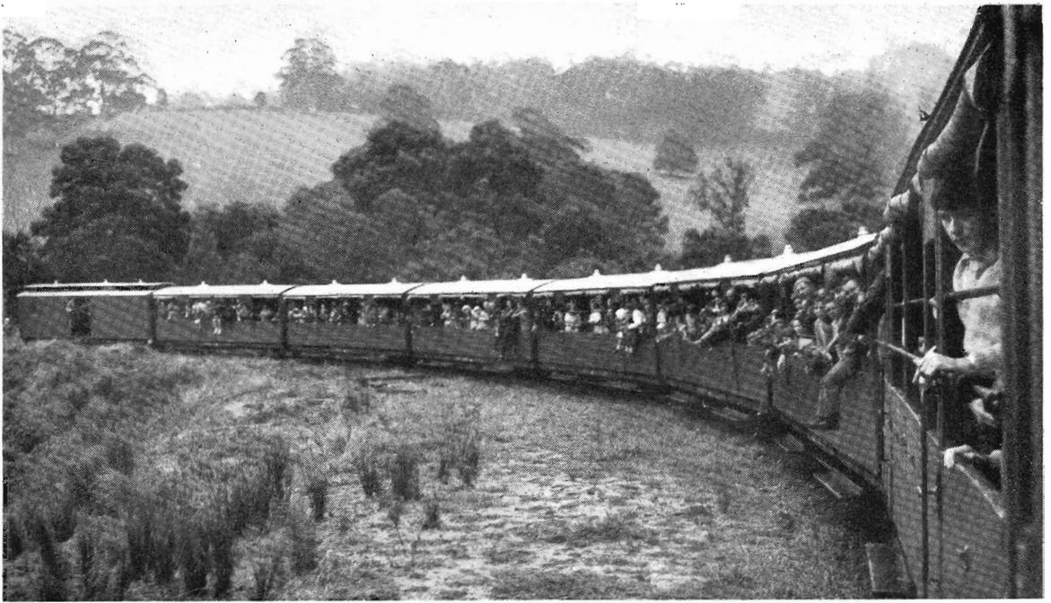
First time past the landslide that, nine years ago, caused the suspension of train services to Gembrook The two chain curve, at 5 m.p.h., is the tightest permitted on a narrow gauge line.
