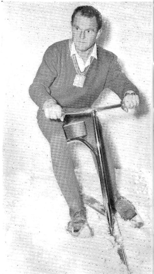
▲ **The latest :** Mr. Ollie Polasek shows how the bicycle is used. Europe's latest snow sport craze, the has a fixed ski at the rear and a moveable ski—by handle-bars—at the front. The rider uses skis to assist control as the bicycle speeds down slopes. It makes its first public appearance at the Mt. Buffalo, this season, where Mr. Polasek is an in
