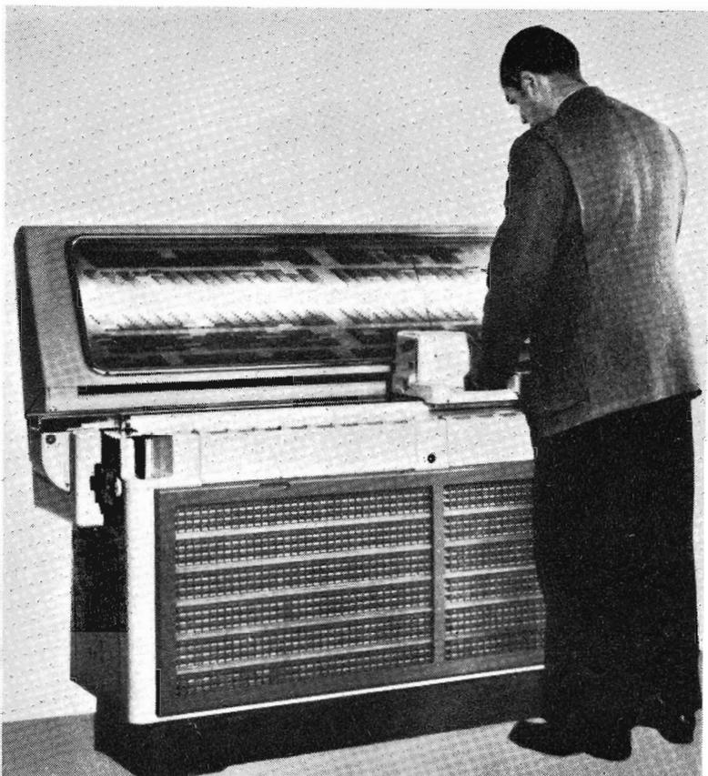
Operator moves the carriage to select a printing plate. At the present time, no machines of this type are operated in Australia, but they are extensively used in Great Britain and on the Continent.
