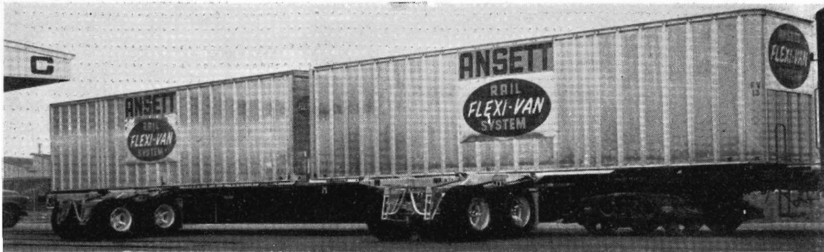
(Above) Double Flexi-Van: The first double Flexi-Van goes into service. The wagon, 75-ft. long, carries two 35-ft. Flexi-Vans and is the first of ten to be used by two of Australia's major transport operators on the standard gauge line.
