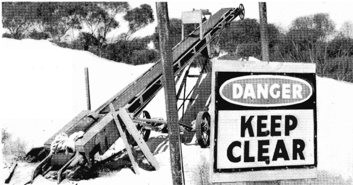
A heap of gypsum with conveyor for loading
