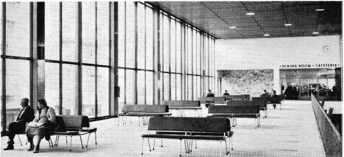
The Waiting Gallery, facing the street. A sound absorbing ceiling, and heavy plate glass in the window wall reduce traffic din. The glass is also tinted to subdue glare.
