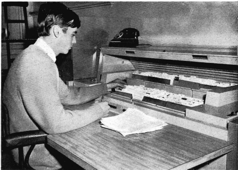
Seated at the unit, Junior Clerk Garry Chandler withdraws a card. The cards are in trays on a "ferris-wheel" carrier that rotates when buttons are pressed. The carrier moves by the shortest route—either up or down—to desk level. As he withdraws a card the operator's hand interrupts a pencil beam of light. This prevents accidental rotation of the carrier.
