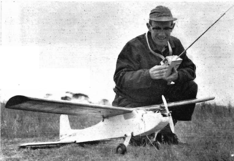
Mr. Blackie with one of his model planes. Powered by a 2½ c.c. glow-plug motor it was made by him out of balsa, 3 ply wood and nylon fabric.
