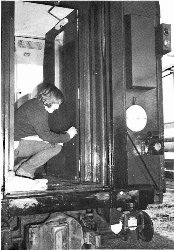
**MODIFIED.** For *The Vinlander* two twinettes and two roomettes from *The Overland* have been painted blue instead of maroon and modified for operation on the Mildura line. Seen renovating the draught seals on the vestibule door is Upholsterer Ian Burns.
