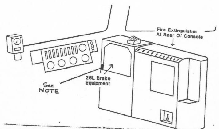
NOTE Dynamic Brake Eircuit Breaker, this circuit Breaker protects the dynamic brake rheostat. MUST BE ON FOR DYNAMIC BRAKE OPERATION from that driving console. The controls in both cabs are identical.
