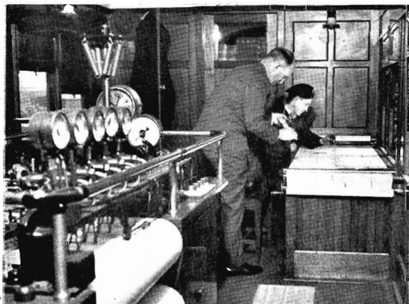
Studying charts during a Dynamometer Car test
