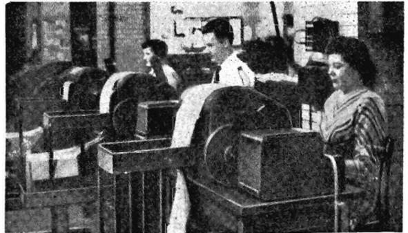
Three teletype machines in operation, with continuous fanfold forms (freight bills) going into receptacles — *Railway Age, U.S.A.*
