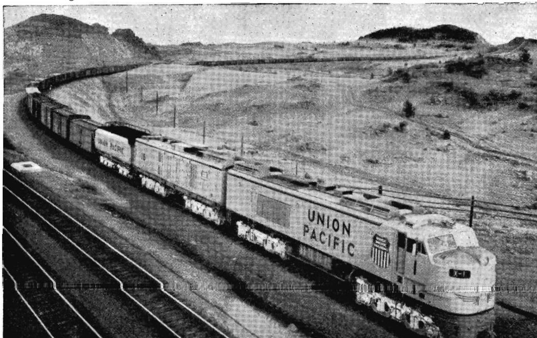
CRESTING a hill in Wyoming, U.S.A. and with the freight vehicles curving away into the distance, this 8,500 h.p., 420-ton two-unit gas-turbine electric locomotive is the pride of the Union Pacific Railroad. On a level track it is said to be able to haul 735 full-loaded freight wagons—a train more than seven miles long. Trailing unit houses the gas-turbine power plant. Total weight of locomotive and fuel tender is 540 tons; length overall, 178 ft. 11½ in., height, 16 ft., width, 10 ft. 10½ in.
