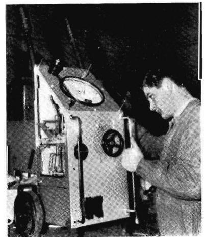
**ANOTHER** recent example of the skill of the Electrical Testing Division's staff : they designed and built this high voltage portable tester for checking electric equipment on suburban carriages. Apprentice Electrical Fitter P. Lawrence is engaged in his work.
