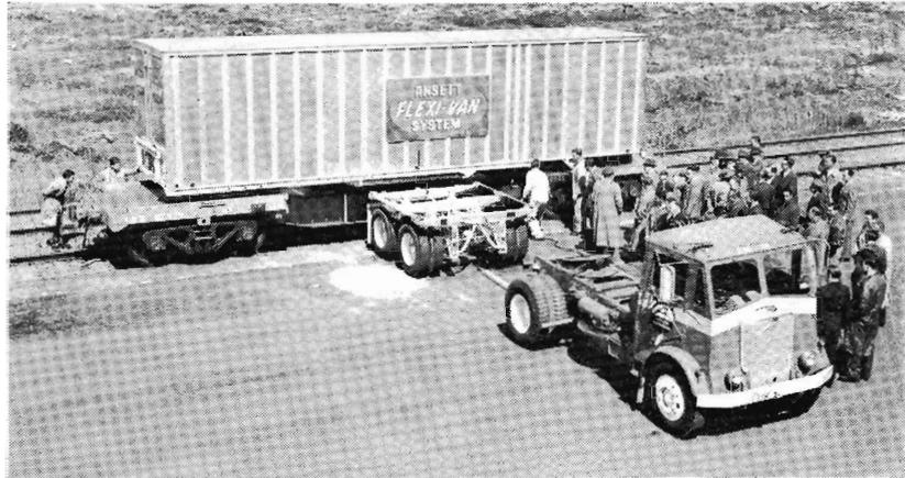
Flexi-van on turntable is being lowered to the self-locking position on rail wagon.
