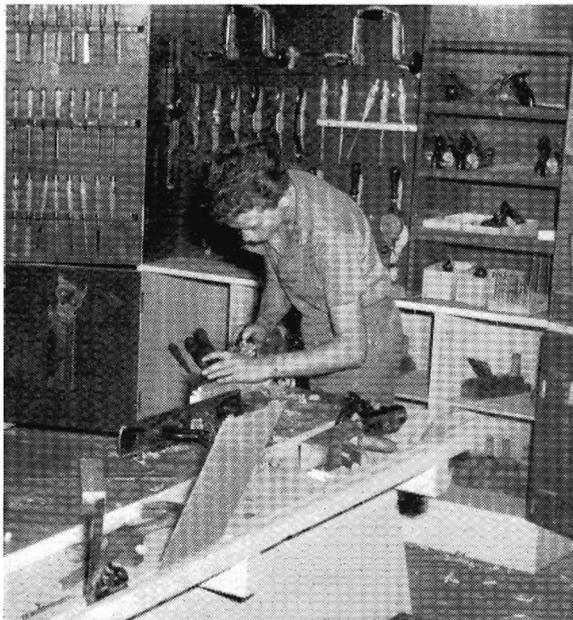
For use in a passenger carriage, a partition is being moulded by Apprentice Car and Wagon Builder, L. Hazelgrove.
