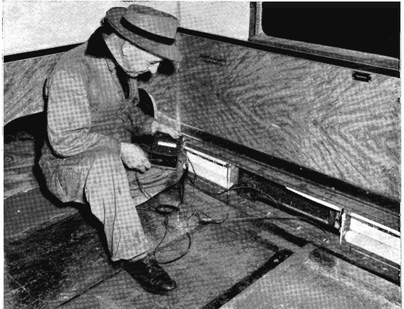
Electrical Mechanic H. B. Holroyd testing heating system in floor of BZ carriage.
